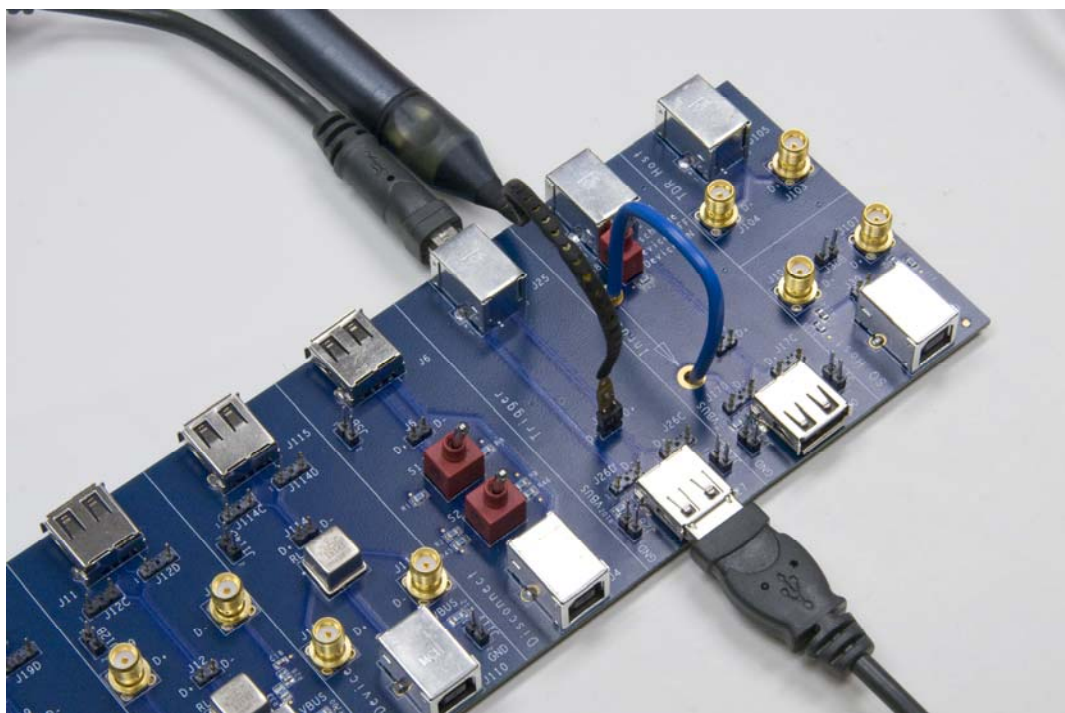
Figure 19. D600ST-SP Connected to the Test Fixture
